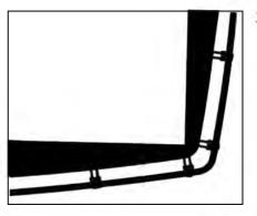
Tighten the screen using the adjustable straps on the right and bottom sides of the movie screen.
