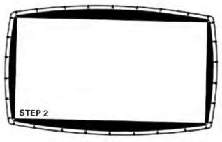
Attach the clips to the frame, starting with the four corners.
