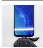
Open the top corners of the device to access the USB-C or microUSB connector & connect to a cell phone
