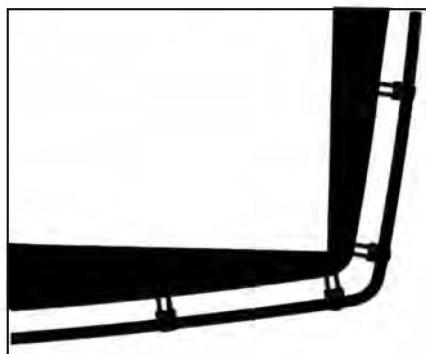
3. Tighten the screen using the adjustable straps on the right and bottom sides of the movie screen.
